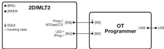
494750\_Wiring Diagramm 2DIMLT2 with OT Programmer
