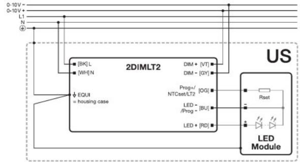
494748\_Wiring Diagramm 2DIMLT2 with NTC
